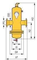
All Spirovents fabricated and stamped in accordance with ASME Section VIII, Division 1 for unfired pressure vessels. Standard rating is 150 psi at 270°F. Consult local sales office for special requirements.
